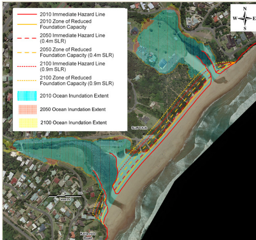
Figure 7: Erosion and Inundation Hazard Mapping at Stanwell Park Beach
